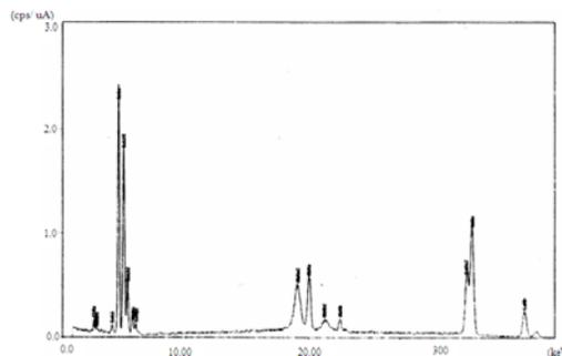
Fig.1 XRF patterns of starting La<sub>0.98</sub> Mn<sub>0.02</sub>O<sub>3</sub> powder at 1000°C
