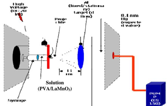
Fig. 5 Schematic diagram of electrospinning set up
