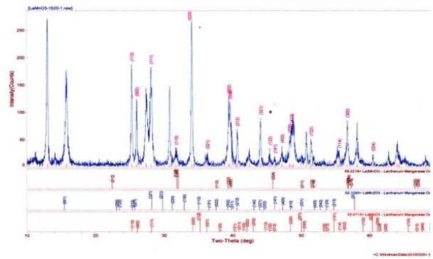
Fig.4 XRD patterns of La<sub>0.98</sub>Mn<sub>0.02</sub>O<sub>3</sub> powders, annealing temperature at 1000°C
