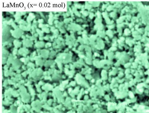
Fig.2 SEM image of lanthanum manganite La<sub>0.98</sub>Mn<sub>0.02</sub>O<sub>3</sub> powder at 1000°C
