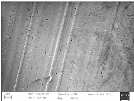
Fig. 7 (b) SEM image of lanthanum manganite  $\text{La}_{0.98}\text{Mn}_{0.02}\text{O}_3$  fibre at  $800^\circ\text{C}$
