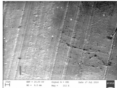
Fig. 7 (e) SEM image of lanthanum manganite  $\text{La}_{0.98}\text{Mn}_{0.02}\text{O}_3$  fibre at  $800^\circ\text{C}$
