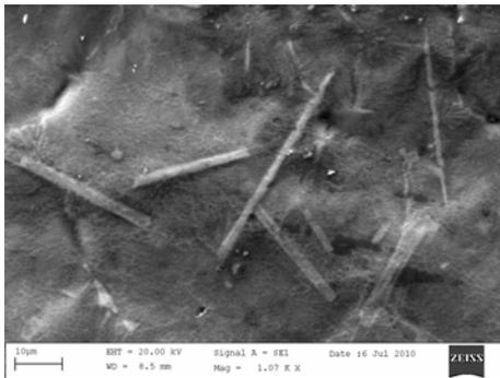
Fig. 7 (a) SEM image of lanthanum manganite  $\text{La}_{0.98}\text{Mn}_{0.02}\text{O}_3$  fibre at  $800^\circ\text{C}$
