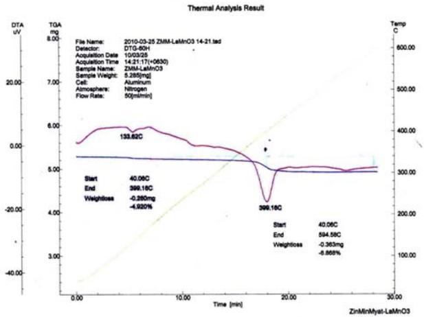
Fig. 3(c) TG-DTA analysis of La<sub>0.98</sub>Mn<sub>0.02</sub>O<sub>3</sub> powder
