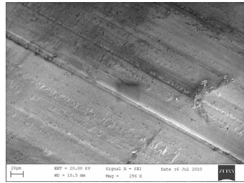
Fig. 7 (c) SEM image of lanthanum manganite  $\text{La}_{0.98}\text{Mn}_{0.02}\text{O}_3$  fibre at  $800^\circ\text{C}$
