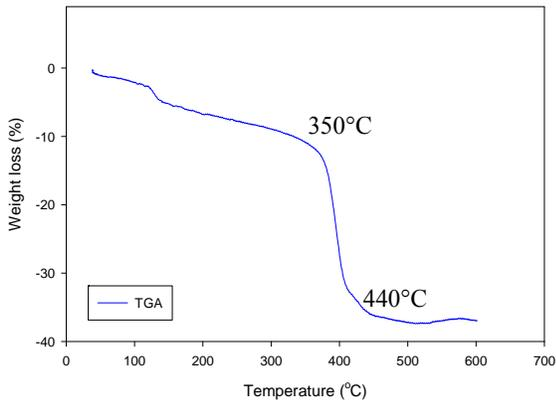
Fig.3 (b) TGA analysis of La<sub>0.98</sub>Mn<sub>0.02</sub>O<sub>3</sub> powder
